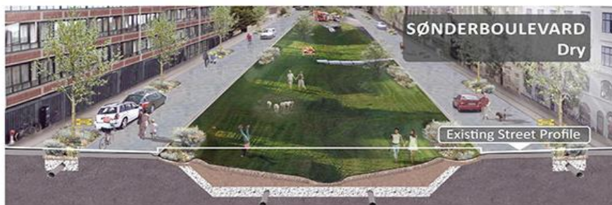
Rain Event Handled within Multi-Functional Tools including Urban Creek, Retention Boulevard, and Boulevard
